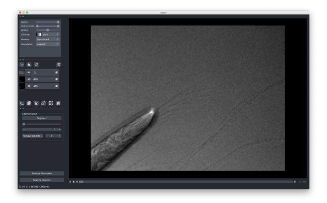
Set the threshold to a reasonable value based on your data. You can use the slider or type in the threshold box to update the threshold interactively. If your images contain small bright objects, you can use the Remove Objects < button to remove objects smaller than the given number.
